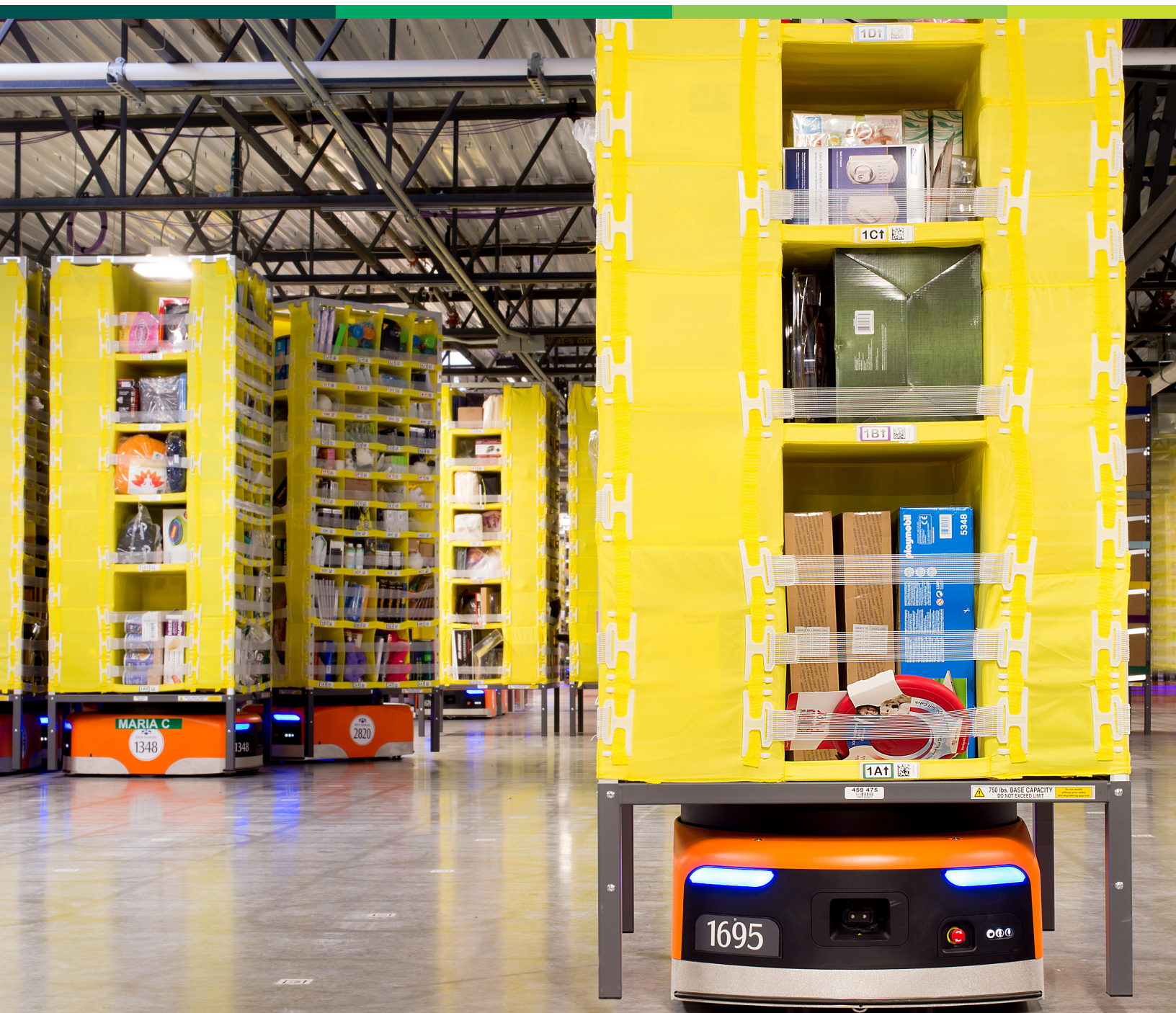
Automated Mobile Robots (AMR) help move goods at Prologis International Park of Commerce, Tracy, California
